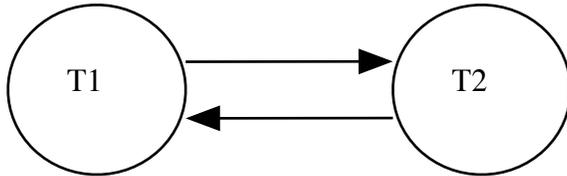
The edge from T1 to T2 arises because T1 must do its read before T2 does its write. The edge from T2 to T1 arises because T2 must do its read before T1 does its write.
