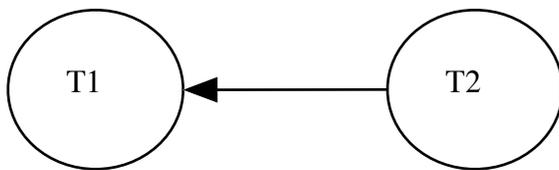
The edge from T2 to T1 arises for two reasons: T2 must do its read before T1 does its write, and T1 reads the value written by T2.
